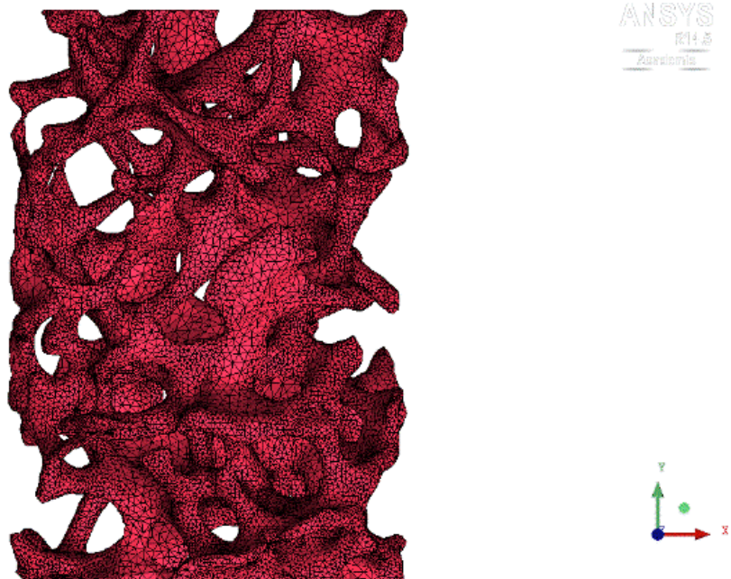
Figure 9. Tetrahedral mesh of a 3D bone model generated in ANSYS ICEM CFD.
